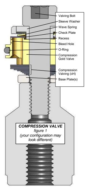
Hold the compression stack up to the light and visually **check for proper assembly**. If there are any problems, disassemble the stack and look for burrs to surface and/or dirt in the valving.
